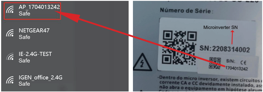
Microinverter SN: 2208314002 Built-in datalogger :1704013242
